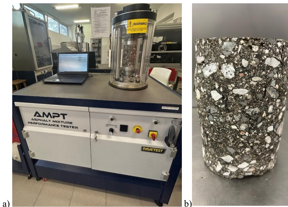
Figure 19 Asphalt Mixture Performance Tester (AMPT) device for Flow Number and Dynamic Modulus testing: a) testing setup with BSM-E specimen, b) BSM-E specimen after testing.
