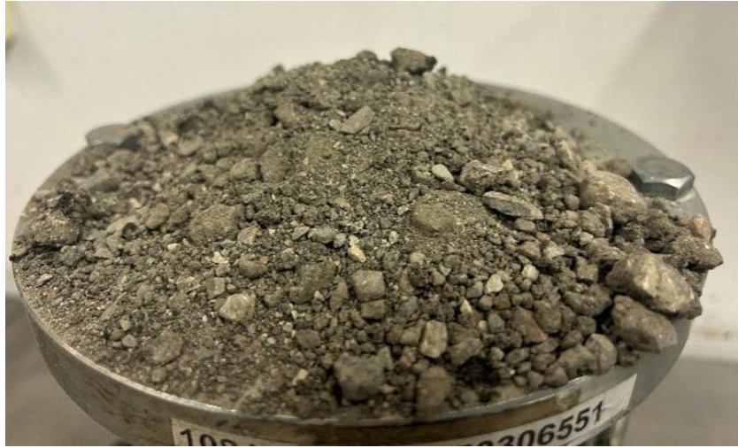
Figure 13 Part of the 100% RAP Marshall sample compacted at 20°C after demoulding
