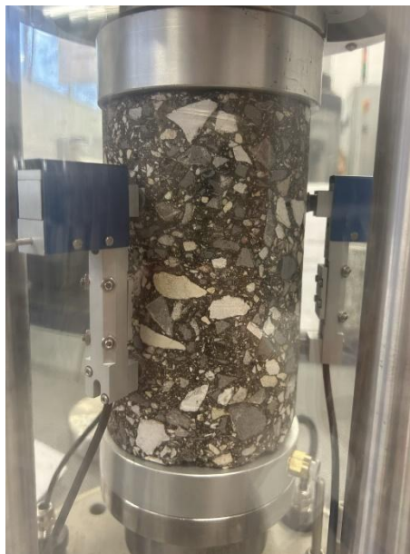
Figure 21 Dynamic Modulus testing setup
